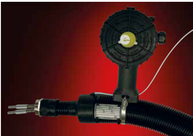
Special analytic heated hose type ELH/2adsbw-100 °C- NW6/8-EX-SP for ex-range with 2 inner liners made of Fluoropolymer NW 6/8 and attached Ex terminal box; type Ex-it-R. Holding temperature: 100 °C
